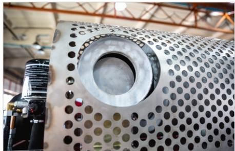
A close-up photograph of a cylindrical spark arrester with a perforated metal mesh, used for filtering exhaust gases.                                           |
